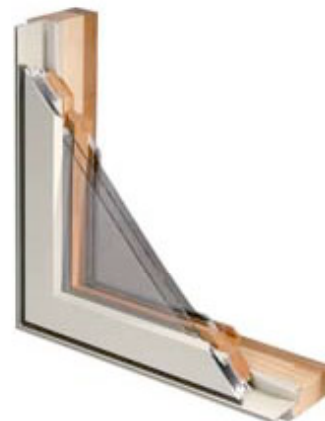
Legends Series C3000 clad replacement casement with 3 1/4" jamb shown in optional oak interior
