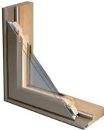
Legends Series C4000 clad 4 9/16" full jamb casement shown in standard western pine interior available in standard sizes for use in new construction or custom sizes for remodeling.
