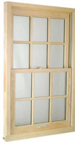
Legends Series DR200 shown with 7/8" simulated divided lite muntins in western pine, permanently applied 6/6 pattern (also available in removable style for easy cleaning)
