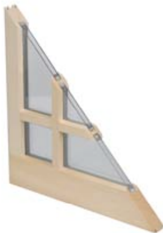
Authentic true divided lite (TDL) with "putty glaze" look 1 1/8" muntin detail shown in western pine with insulating glass and warm edge super spacer glazing (exterior view).
