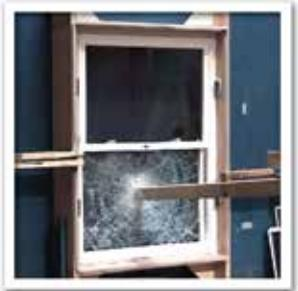
AIP Windows carry a DP-50 rating in accordance with the American Architectural Manufacturers Association's 101 standard for air, water and structural wind load testing.
