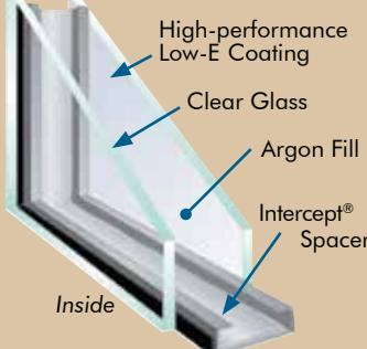
Above values are for a Barrington double-hung window with Solar Low-E, featuring single-strength glass, Intercept spacer, argon gas, and without grids.
