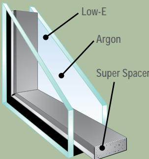
Above values are for a Pro double-hung window with Low-E, featuring single-strength glass, Super spacer, argon gas, and without grids.
