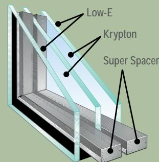
Above values are for a Pro double-hung window with Ultimate Glass, featuring triple-strength glass, Super Spacer, krypton gas, and without grids.
